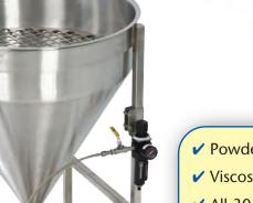
includes a 3.5 cubic foot powder hopper, ergonomic waist-high work table, sanitary powder suction pump, powder valve, vacuum gauge, vacuum regulator
