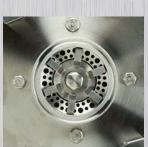
shearing action and "pre-mixes" the materials prior to entering the secondary stage. Particle and droplet size reduction down to 5 - 7 microns is typical in this stage.
